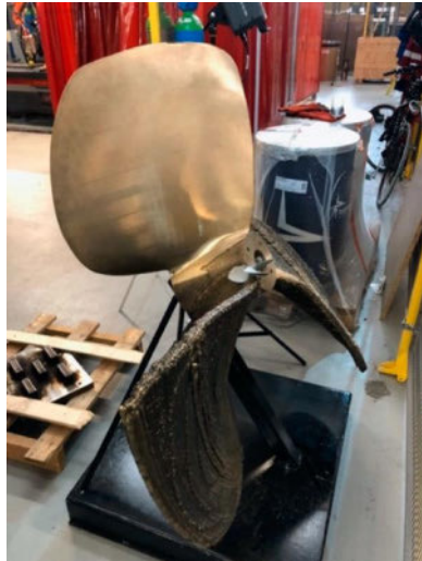
Figure 1. Propeller produced by WAAM (wire arc additive manufacturing).
